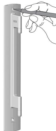
3. Drill mounting holes (only required for wall mounting).
